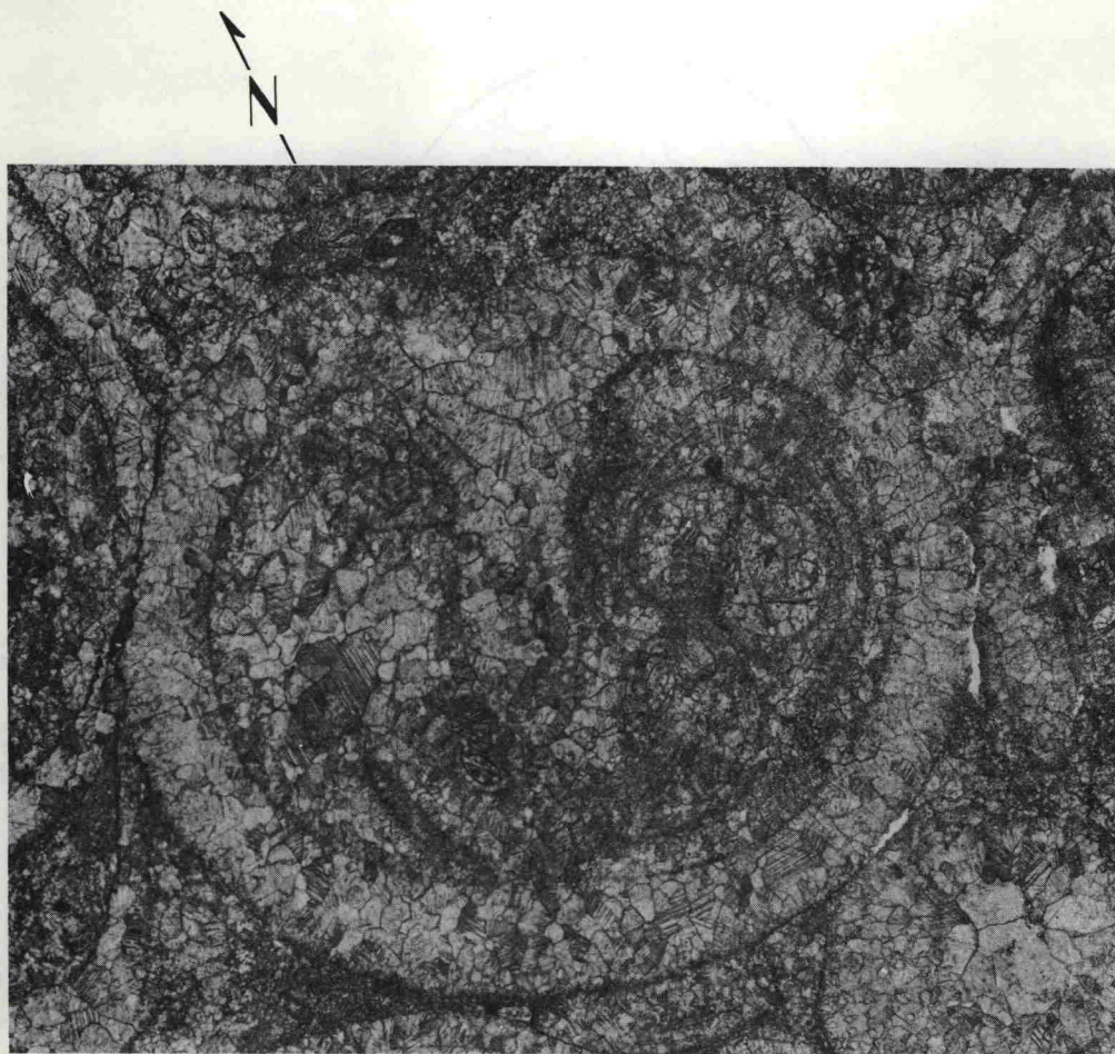
Fig. 28—Photomicrograph of a transverse section through a gastropod. Plane of the photomicrograph is also parallel to bedding. North is as indicated after the bedding is rotated to the horizontal. East-west diameter of the gastropod is approximately 4 mm (from Friedman and Conger, Ref. 112, Plate 1).
